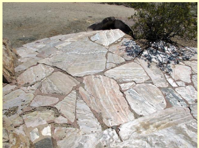
A muscovite rich phyllite, mined in the Phoenix Mountains and used as flagstone
