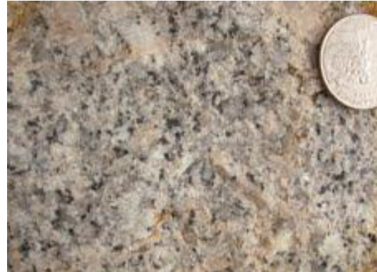
Granite from the Walker Butte Granite Quarry near Florence, gray is quartz, pink is microcline, white is plagioclase, and black is biotite.
