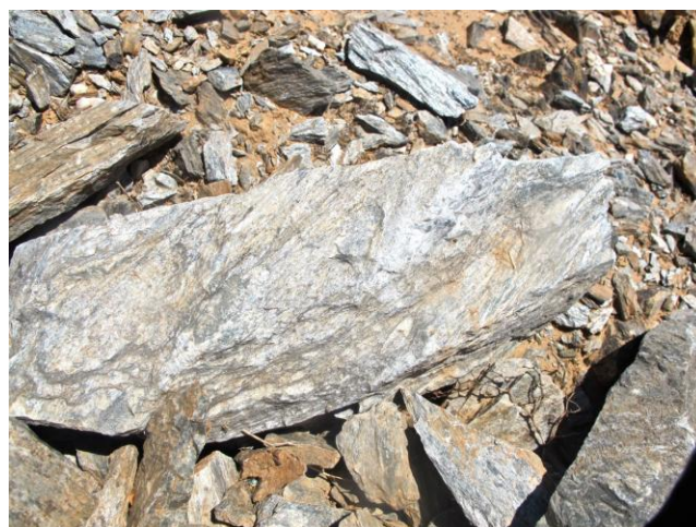
Phyllite, you can almost see individual minerals, but it is still very fine-grained. It does not break smooth like slate.
