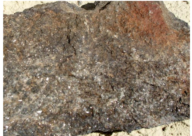
Pinal schist (quartz mica schist) from the San Tan Mountains, note the rough surface and the reflections from the mica crystals.
