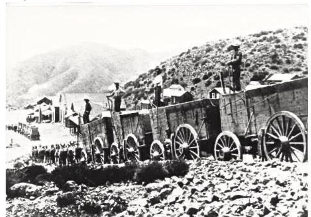
Wagons carrying ore from the Silver King Mine to Pinal. Note steel rim wheels, Arizona Geological Survey photograph
