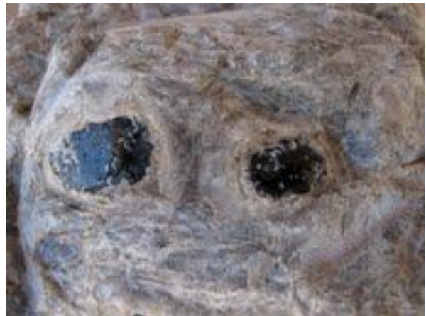
Obsidian in perlite from Superior, AZ (the whole specimen was originally obsidian, but has changed to perlite by hydration).
