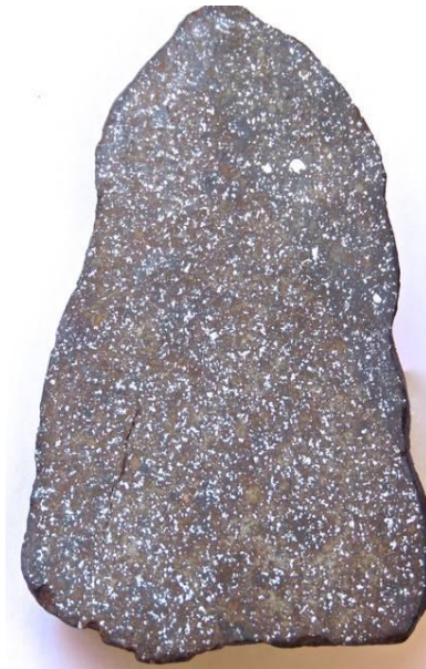
Slice of stony meteorite showing nickel-iron from Plainview, Texas. This meteorite has about 26% metal.
