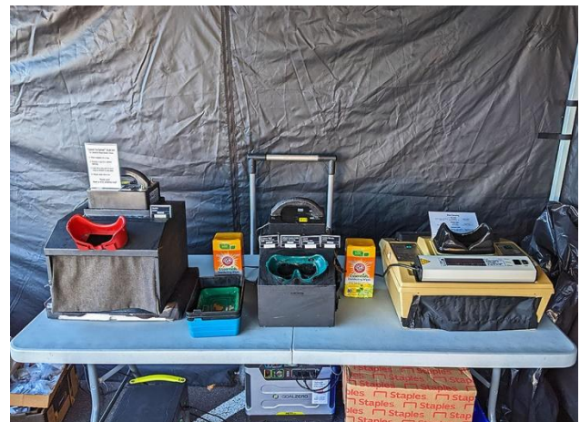
Arrangement of Fluorescent Viewing Cabinets
