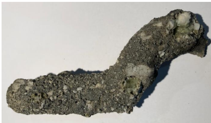
Fulgurite from near Colossal Cave, Pima County, Arizona - Note the green glassy areas.
