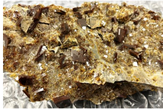
Close up of barite from the Magma Mine, Superior, AZ showing tabular crystal form.
