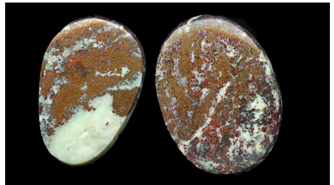
Campbellite, a lapidary material named after the Campbell Mine in Bisbee, It is a mixture of copper, cuprite, and other copper minerals.
