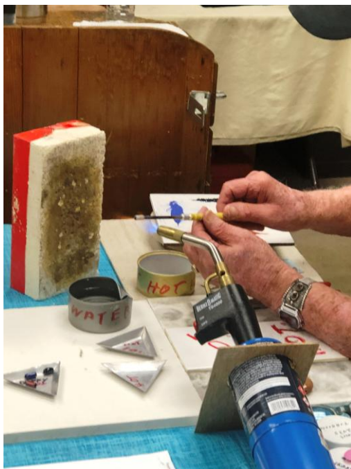
Soldering boards, fire brick, propane tank with torch and containers for water and finished beads.
