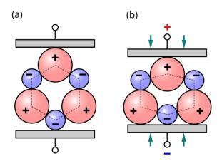
Simplified Model of a Quartz Crystal Between Two Electrodes
