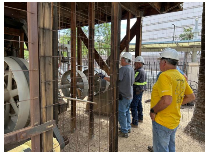
Millmen working on the belt of the Swallow Mine 5-stamp mill.
